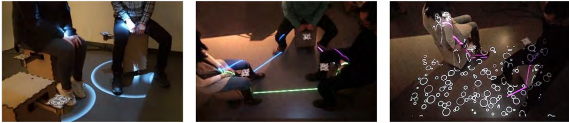
Figure 1: Three interactions of SocialStools . (A) Visualization of personal space; (B) Changing volume, pitch, and timbre of sound output by distance between stools; (C) Changing of shapes and colors of bubbles on the floor by angular orientation of stools.
